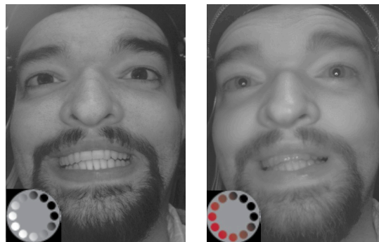
Fig. 4. Comparison of face lit by (left) visible and (right) near infrared gradients.
