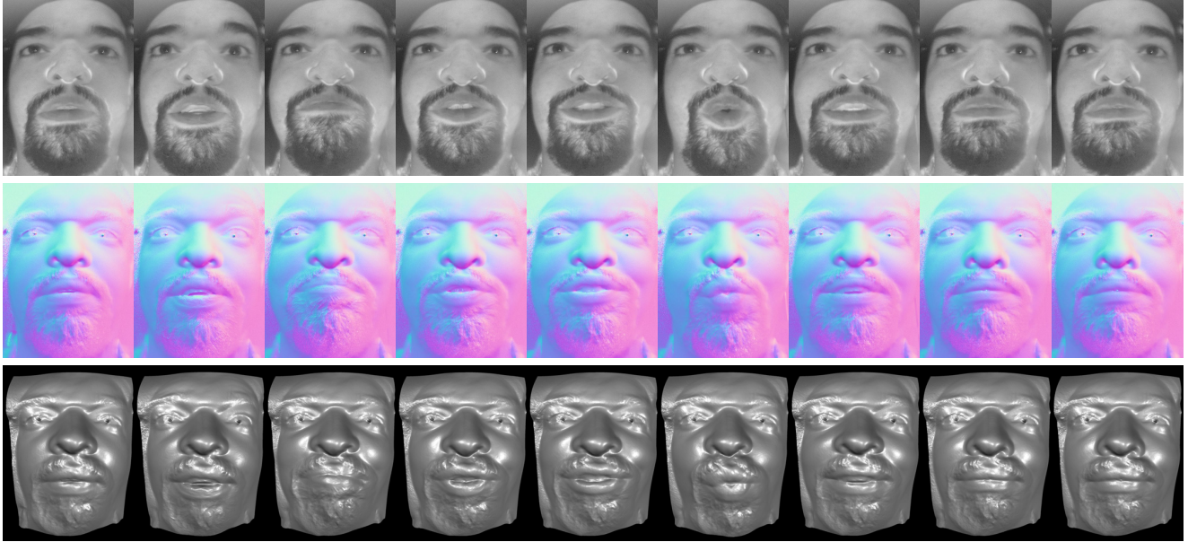
Fig. 8. Results showing every 18th frame from a performance captured under single LED illumination. (row 1) Surface albedo recovered using photometric stereo, (row 2) surface normals with XYZ encoded as RGB, (row 3) integrated surface geometry.
