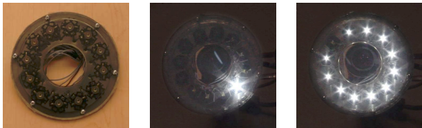
Fig. 2. (left) The LED ring, (center) a single-LED pattern, (right) a gradient LED pattern.
