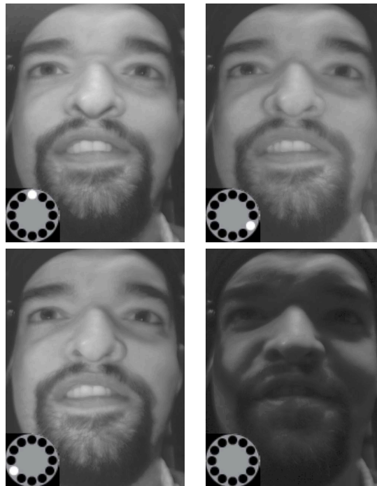
Fig. 3. Four time-multiplexed illumination conditions using single visible LEDs, showing three lighting directions and an image of only the ambient light in the environment
