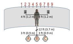
**Fig. 1.** Three loudspeakers, located behind a perforated (sound transparent) screen, provided audio to the left of the projected virtual human, at the center, or in stereo. Participants stood at positions: A, B, or C.
