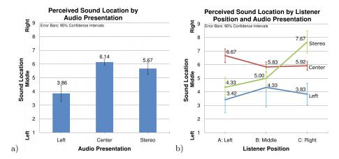
**Fig. 2.** a) Significant differences in perceived location were observed for audio conditions. Localization of speech from the left loudspeaker clearly differed from center and stereo presentations. b) A significant interaction effect on perceived location was observed for listener position and the stereo audio condition. Listeners on the left localized the stereo sound to the left, while listeners on the right localized it to the right.
